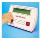
Selecting the desired room – to select the room you wish to speak to, turn the SELECT control clockwise or anticlockwise. This will allow you to scroll through the rooms on the system, until the name of the room/resident you wish to communicate with is on the top line of the display. In the example shown on the left, BEDROOM 21 is being selected.
