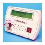
**To call and speak to a room** – All rooms on the system can be contacted providing the call point in the desired room is not already in use. Only available call points will appear in the selection list. Rooms may be contacted independently, regardless of other system activity.
