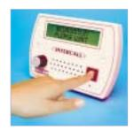
The privacy beep – with the desired room showing on the top line, press and release the TALK button as shown on the left. There will be a small delay while the room is contacted, before the privacy beep is sounded in the room and at the Room Communicator. While the room is being contacted, the screen will show PLEASE WAIT on the lower line of the display.
