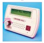
**Broadcast or tannoy messages to all rooms** – the Room Communicator can be used to make announcements to all rooms. Call Points can be contacted regardless of other system activity, providing the speech channel is not in use.
