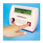
To open the speech channel, the TALK button is pressed when the desired room is showing on the top line of the LCD Display. The operator must press and hold the TALK button while speaking to the room, and release the talk button to allow the resident to reply. Pushing the SELECT control closes the intercom channel.
