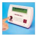
Closing the speech channel – when the conversation is complete, the intercom may be closed by pressing the SELECT button once, as shown on the left. This will reset the unit and close the intercom channel.
