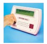
**Selecting another room** – once the speech channel has been closed and the room is again showing on the top line of the display, another room can be selected using the **SELECT** control as previously described. Alternatively, if the **SELECT** control is not operated for 10 seconds, the unit will return to the default text **INTERCALL 700**.
