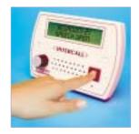
Opening the speech channel – after the privacy beep has sounded, the intercom channel will be open and the call point will be able to speak to the Room Communicator. Press and hold the TALK button while speaking to the room, and release to allow the room to speak. While the speech channel is open the words SPEECH OPEN will be showing on the lower line of the display.
