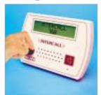
There are two simple controls on the front panel, the rotary and push **SELECT** control and the **TALK** button. Rotating the **SELECT** control scrolls through the list of rooms on the LCD screen. Rotating the control clockwise will move forwards through the list, while rotating anticlockwise moves backwards through the list.
